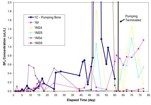
SF<sub>6</sub> Tracer breakthrough in pumping and monitoring wells
