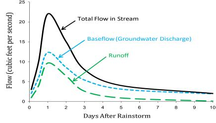
Post-storm hydrograph. Baseflow and runoff components were separated using environmental tracers (e.g., <sup>18</sup>O, <sup>2</sup>H, TDS, silica)
