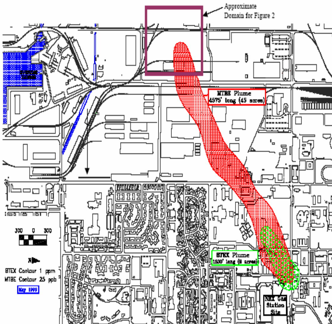
Figure 3-1. MTBE plume (May 1999) at the Naval Base Ventura County, Port Hueneme, California (NAVFAC 2001)
