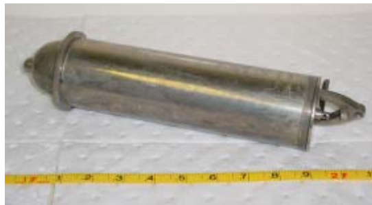
Figure 5.27 Bacon Bomb Sampler (Photograph by J. Schoenleber)
