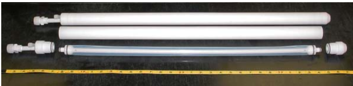
Figure 5.4 Example of a Teflon® constructed bladder pump, complete (top) and exploded version illustrating internal Teflon® bladder (Photograph by J. Schoenleber)
