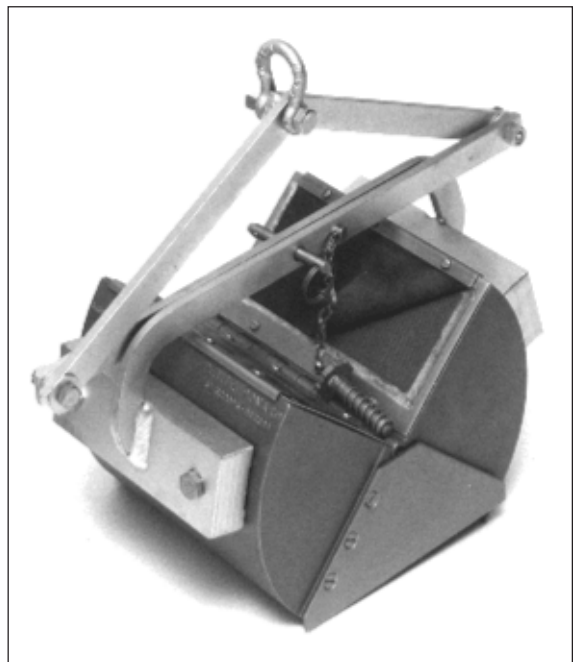
Figure 5.36 Ponar Dredge. Illustration published with permission of Wildco®
