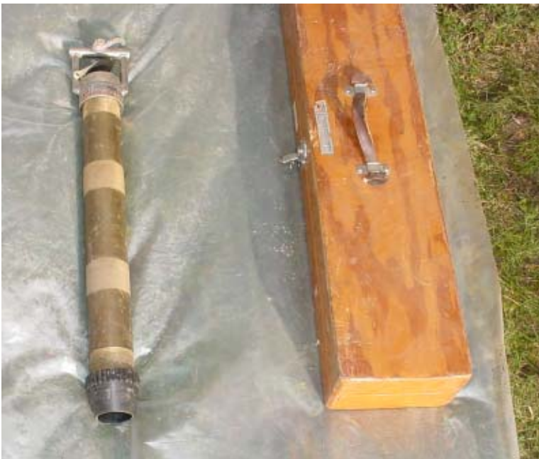
Figure 5.42 Hand Corer (Photograph by J. Schoenleber)
