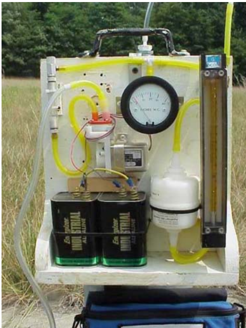
Figure 9.13A Purge pump with flow control and vacuum gauge, Photographed by C. Van Sciver
