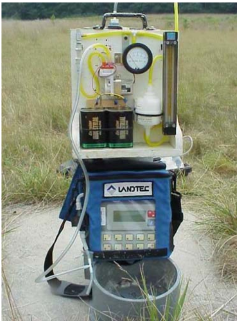
Figure 9.13B Purge pump with DRI inline, Photographed by C. Van Sciver
