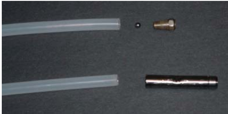
Figure 5.13 Two styles of foot check valves offered by Geoprobe® for narrow diameter temporary well points (Photograph by J. Schoenleber)
