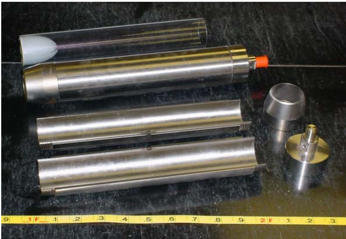
Figure 5.33 Soil Coring Device (Photograph by J. Schoenleber)
