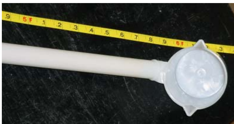
Figure 5.19 Pond Sampler (Photograph by J. Schoenleber)
