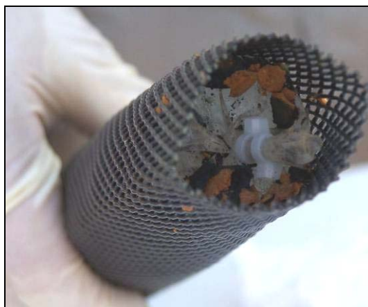
Figure 5-7. Top of RGC sampler showing deposits of large black and orange particles.
