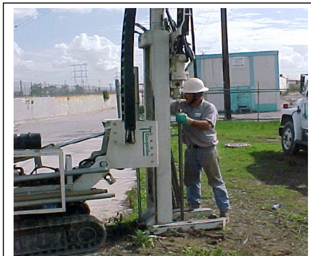
Figure 1. Investigating Subsurface Contamination at Pemaco with a Direct Push Rig
