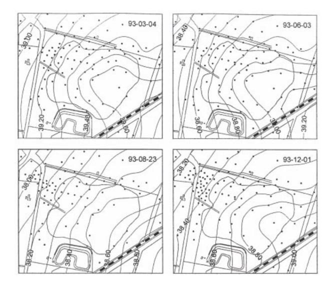
Figure 3. Mounding of the leachate-groundwater table below Grindsted Landill shown as isopotential contours for the landfill and surrounding area at 4 different seasons during 1993. Modified from Kjeldsen et al. (1998).
