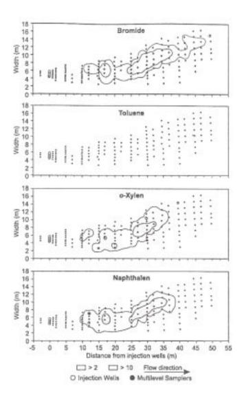
Figure 5. Observed clouds of bromide, toluene, o-xylene, naphthalene after 649 days. Bromide in g/m<sup>2</sup>, xenobiotics in mg/m<sup>2</sup> (From Rügge et al., 1999a).
