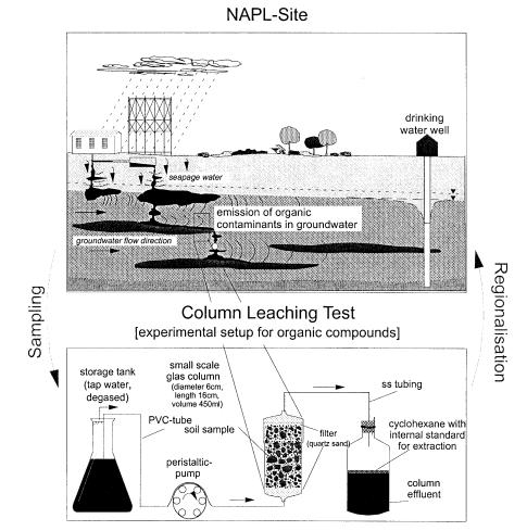
Figure 2. The emission from a contaminated site (location, size and strength of source) is commonly performed on the basis of *soil sampling* and *leaching tests*. Even though the leaching test procedures are being improved considerably and also standardised, the regionalisation of the test results is considered highly uncertain.
