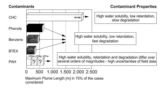
Figure 4. Typical plume length for different contaminants: Natural attenuation is effective for all (organic) compounds but quantification requires site-specific data.
