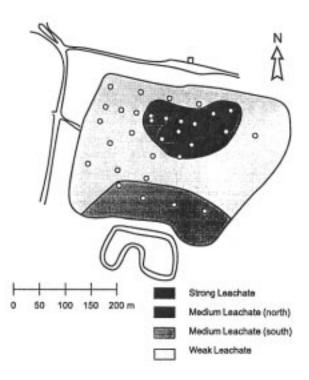
Figure 2. Division of the landfill into four areas with different leachate (Kjeldsen et al., 1998a).
