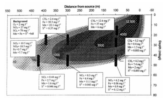
Figure 1. Schematic cross section of phenol plume (mg.l<sup>-1</sup>) beneath site with selected groundwater quality data. Borehole positions and screen length are shown in black.
