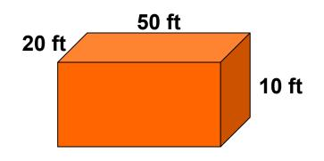
10,000 cf impacted by DNAPL 30% porosity = 3,000 cf TREAT 10% to 30% of porosity = 300 to 900 cf EVZI
