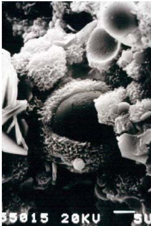
Figure 3.8: PFA spheres covered with hydration products (Photograph courtesy of Colin Hills).
