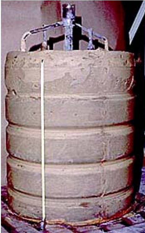
Figure 6.8: In-drum S/S of radioactive waste processing (Photograph courtesy of BNFL)
