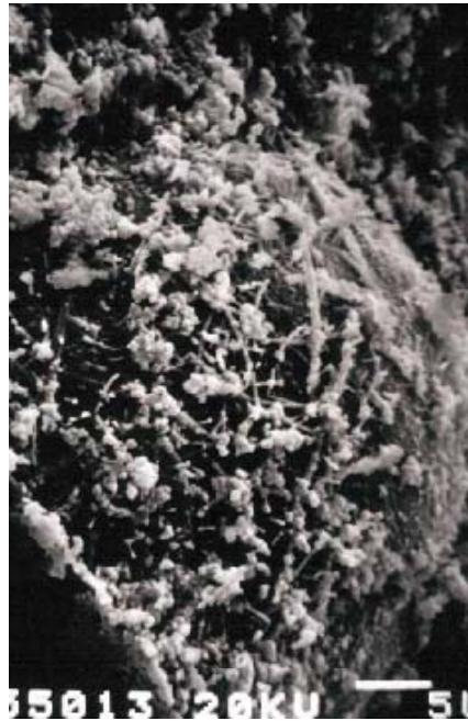
Figure 3.1: Particle of heavy metal-contaminated material, derived from treatment of metal plating residues, encapsulated in a PC matrix (photograph courtesy of Colin Hills).
