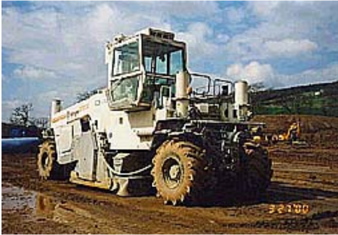
Figure 6.6: A direct mixing plant (rotovator) (Photograph courtesy of the machine manufacturer, Wirth)
