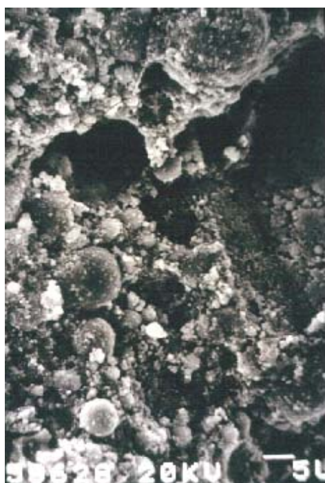
Figure 4.3: An S/S waste form where interference effects can be observed (photograph courtesy of Colin Hills).
