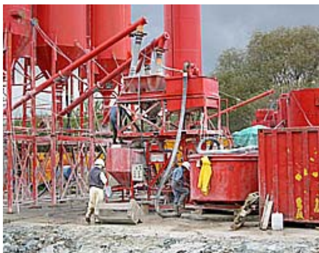
Figure 6.3: Close-up of the above illustrating the reagent delivery systems (Photograph courtesy of Colin Hills)
