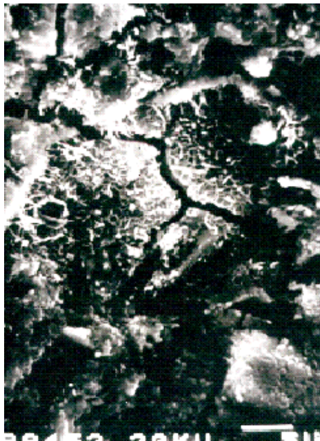
Figure 3.3: Secondary electron photomicrograph of a 'Hadley' grain formed in PC paste (Photograph courtesy of Colin Hills).
