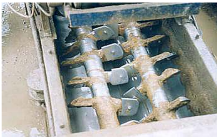
Figure 6.12: Twin shaft Pugmill mixer with exposed mixing blades during inspection (Photograph courtesy of British Cement Association)
