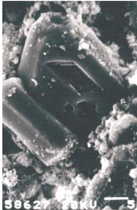
Figure 4.4: Gypsum crystal formation in an S/S waste form (photograph courtesy of Colin Hills).
