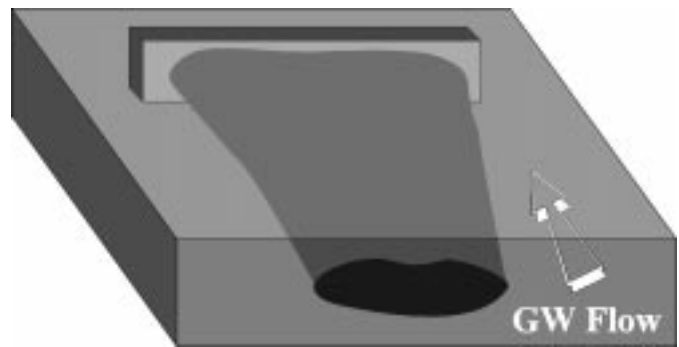
Figure 3b. Plume capture by a continuous trench system. The plume moves unimpeded through the reactive gate.
