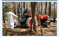
Deploy direct-push equipment rather than hollow-stem auger drill rigs for sampling, to minimize land and ecosystem disturbance. Kerr-McGee Navassa Superfund Site, North Carolina
