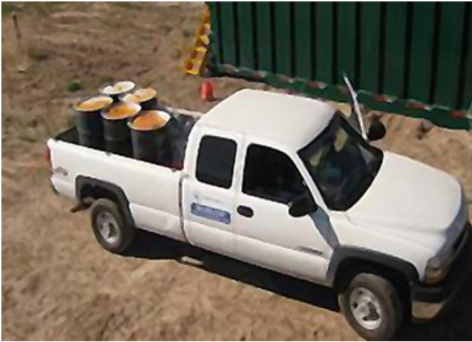
Product Recycling: Recovered product accumulating in the onsite AST is transferred to 55-gallon industrial containers for transfer to a recycling facility in Phoenix, Arizona.
