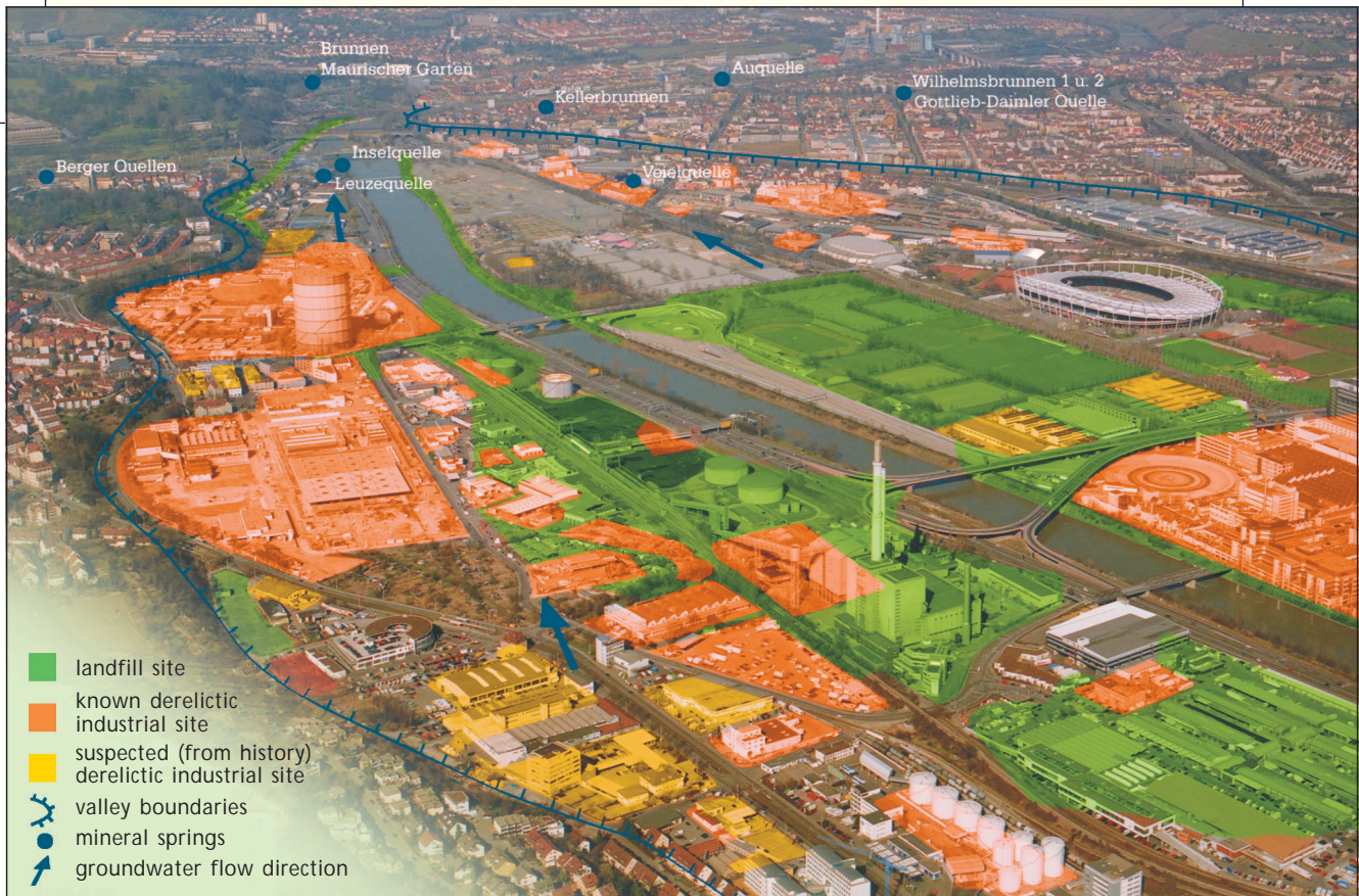
Fig. 1: Project area Stuttgart with complex contamination patterns
