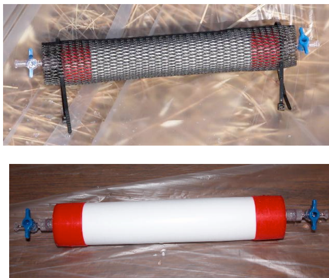
Figure 4 – RPPS with (top) and without (bottom) mesh covering used to secure sampler to deployment rope.
