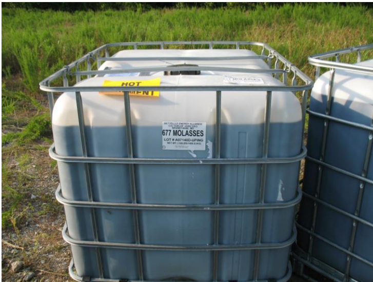
Figure 5-25 Molasses tanks. Three tanks with 3100 lbs of molasses each were used for the injection
