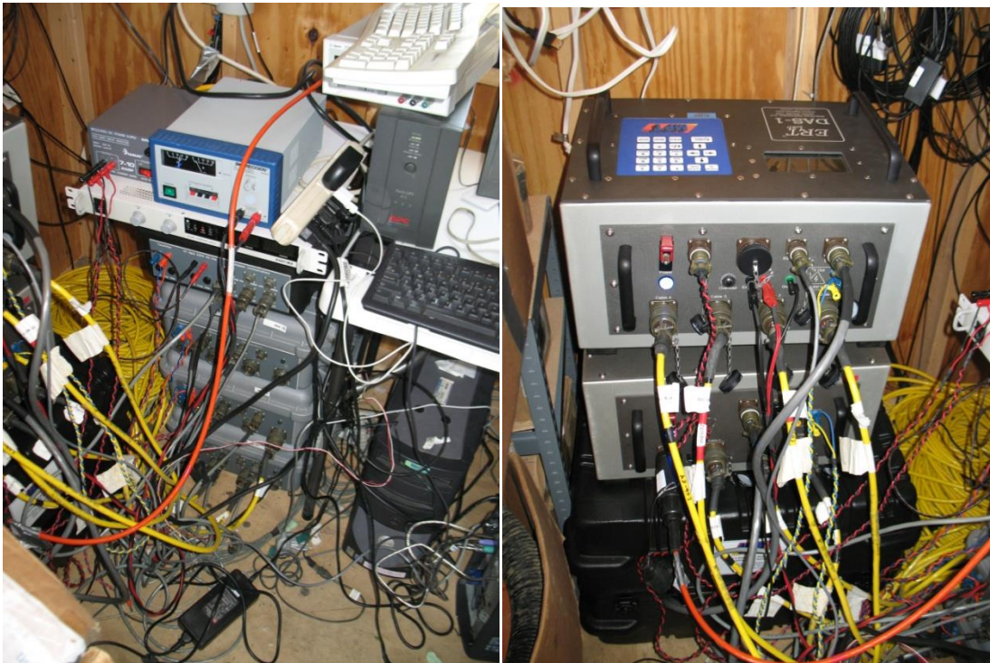
Figure 5-8 Resistivity hardware: left single channel system. Right multi channel system. Both systems use the same electrodes. The multichannel system was used to monitor the second injection
