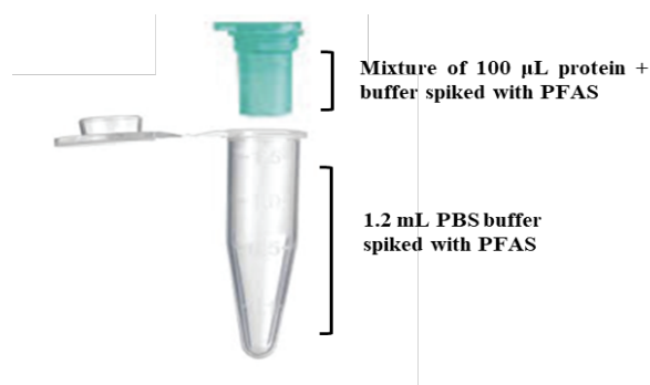
Figure 1. The schematic of equilibrium dialysis experiment
