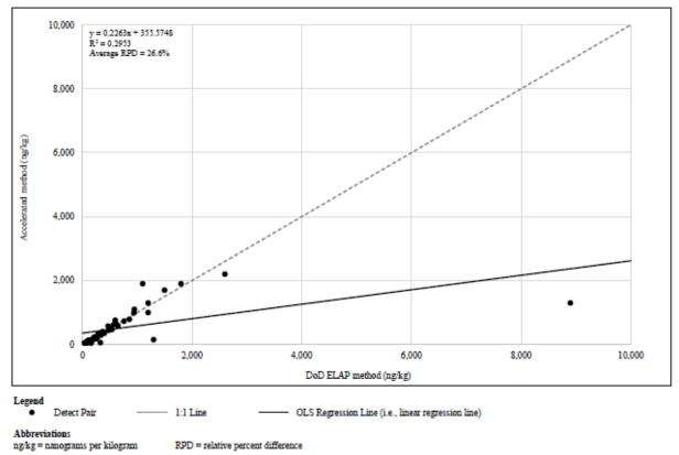
Figure 7-2Q. Secondary PFAS Compound - PFHxS - Soil - Detect Pair X-Y Scatterplots
