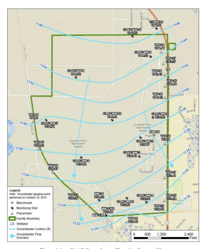
**Figure 4-1.** GAAF Groundwater Elevation Contour Map ESTCP Grayling Army Airfield. Grayling, Michigan Source: AECOM, Site Inspection Report, Camp Grayling Army Airfield, Michigan
