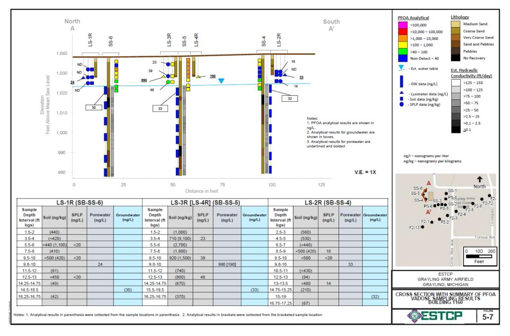
Figure 5-7. Cross Section with Summary of PFOA Vadose, Sampling Results Building 1160
