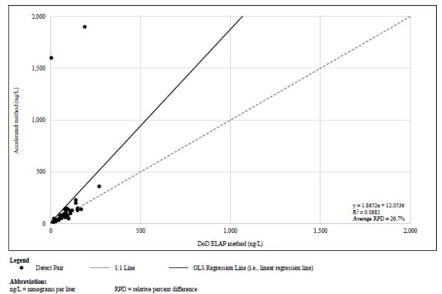
Figure 7-2D. Secondary PFAS Compound - PFHpS - Groundwater - Detect Pair X-Y Scatterplots
