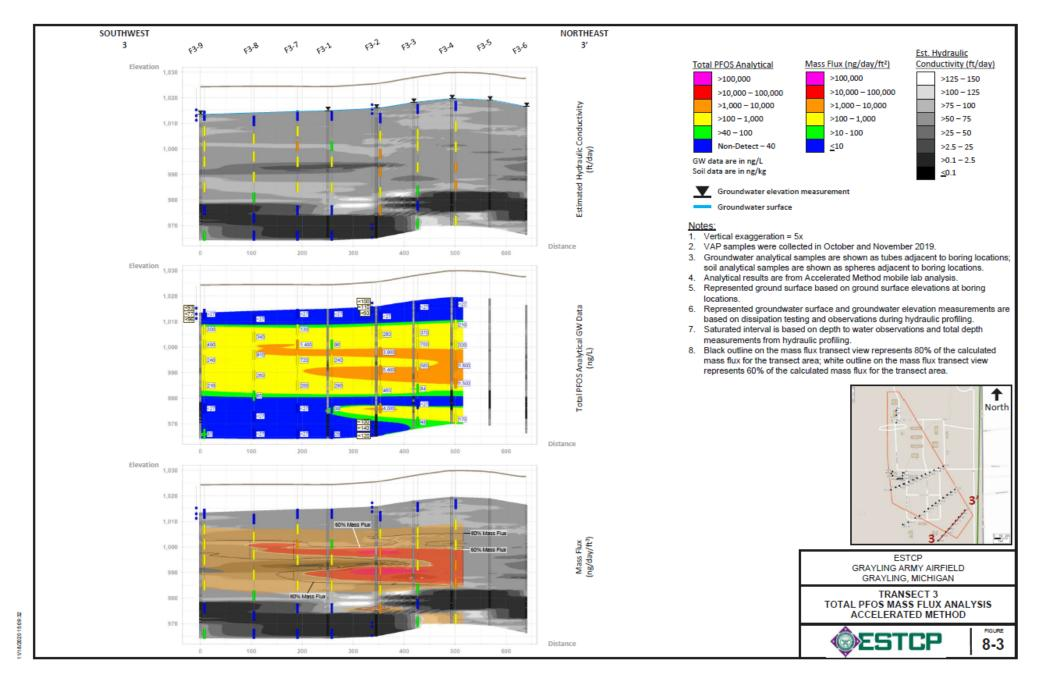
Figure 8-3. Transect 3 Total PFOS Mass Flux Analysis Accelerated Method
