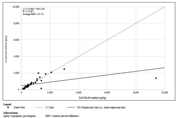
Figure 7-2S. Secondary PFAS Compound - Total PFHxS - Soil - Detect Pair X-Y Scatterplots
