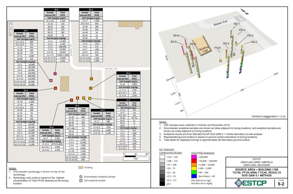
Figure 5-2. Source Area – Building 1160 Total PFOS Analytical Results DoD QSM 5.3 Method
