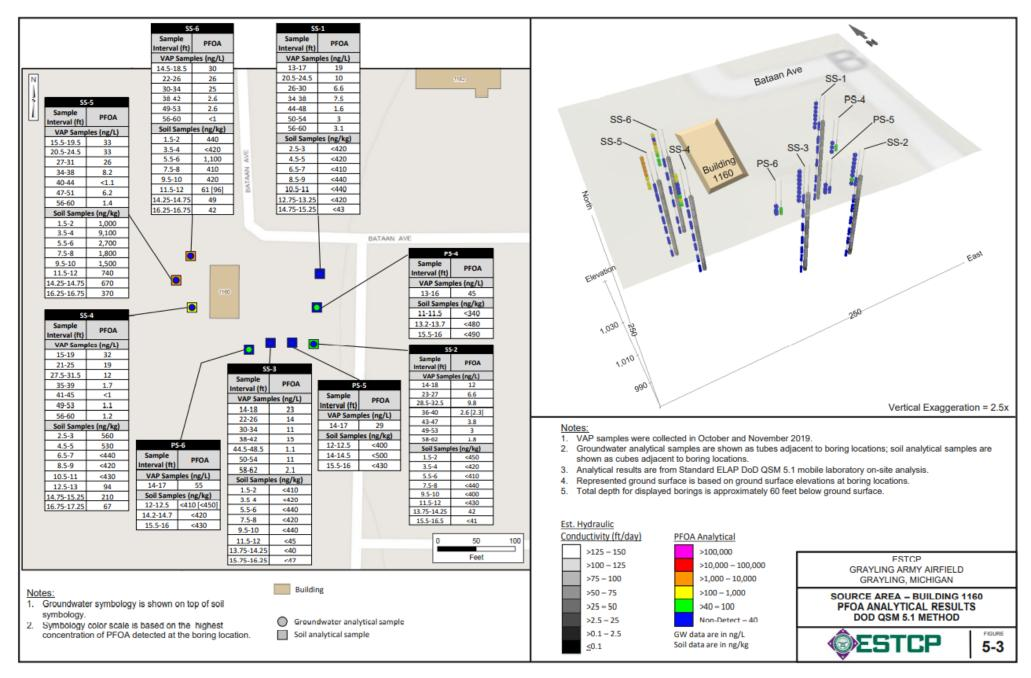
Figure 5-3. Source Area – Building 1160 PFOA Analytical Results DoD QSM 5.1 Method
