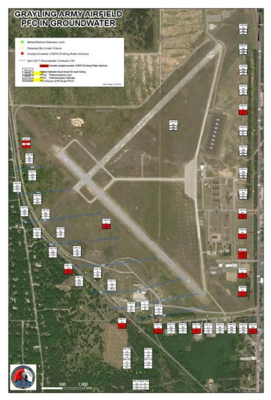
Figure 4-2. GAAF Perimeter Groundwater Sampling Results ESTCP Grayling Army Airfield. Grayling, Michigan
