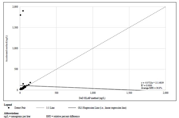
Figure 7-2K. Secondary PFAS Compound - PFPeS - Groundwater - Detect Pair X-Y Scatterplots
