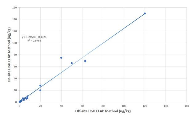
Figure 6-2. On-site vs. Off-site Soils Data, ug/kg
