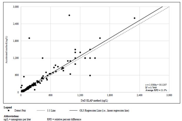
Figure 7-2H. Secondary PFAS Compound - Total PFHxS - Groundwater - Detect Pair X-Y Scatterplots
