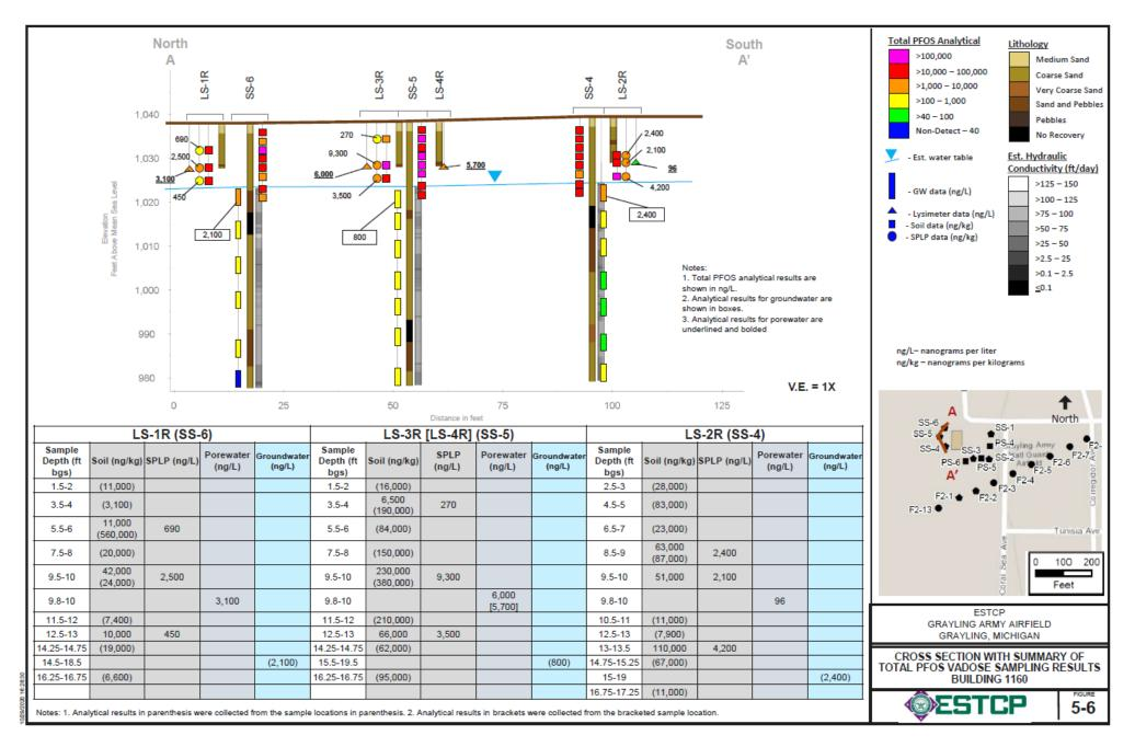
Figure 5-6. Cross Section with Summary of Total PFOS Vadose, Sampling Results Building 1160
