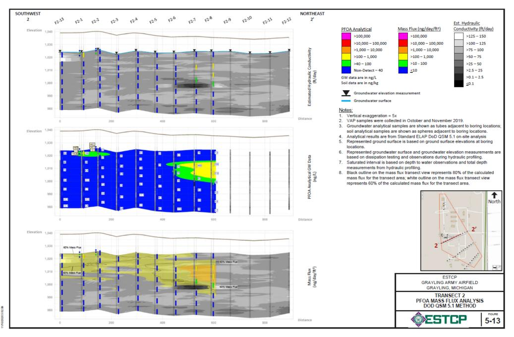
Figure 5-13. Transect 2 PFOA Mass Flux Analysis DoD QSM 5.1 Method
