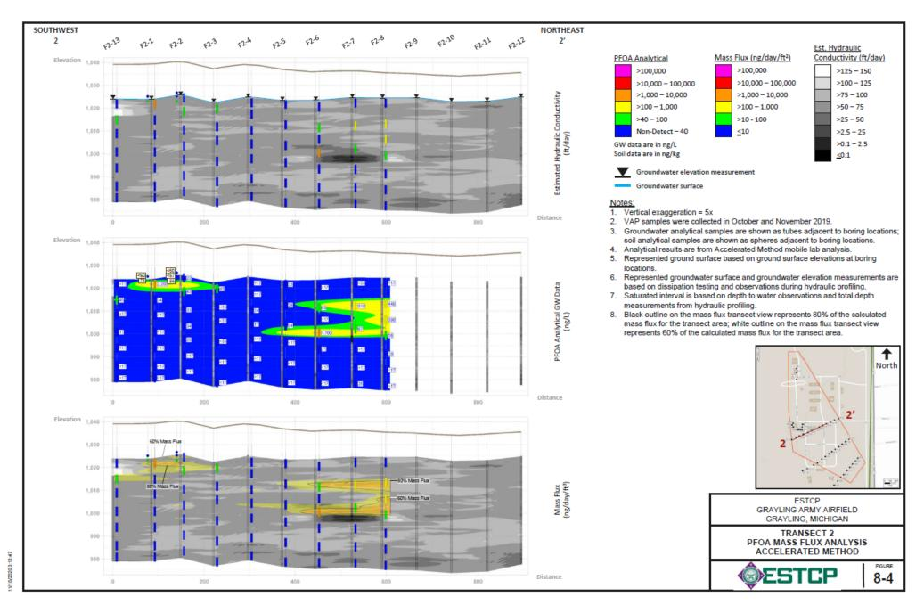
Figure 8-4. Transect 2 PFOA Mass Flux Analysis Accelerated Method
