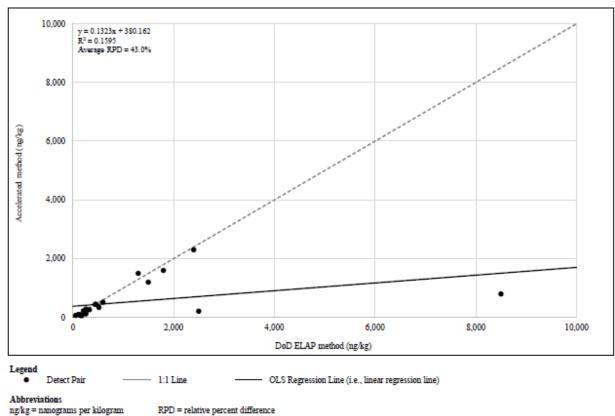
Figure 7-2T. Secondary PFAS Compound - PFNA - Soil - Detect Pair X-Y Scatterplots
