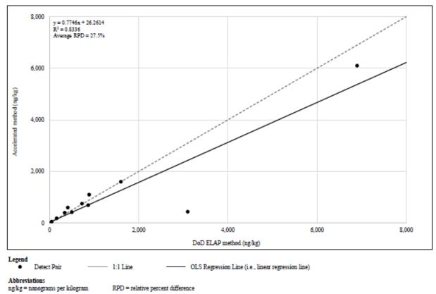
Figure 7-2L. Secondary PFAS Compound - 6-2FTS - Soil - Detect Pair X-Y Scatterplots
