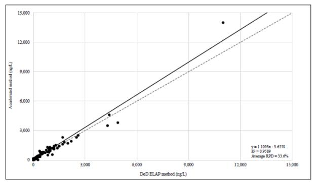
T-PFOS - Groundwater - All Detect Pairs
