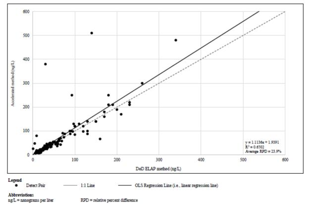
Figure 7-2G. Secondary PFAS Compound - Br-PFHxS - Groundwater - Detect Pair X-Y Scatterplots
