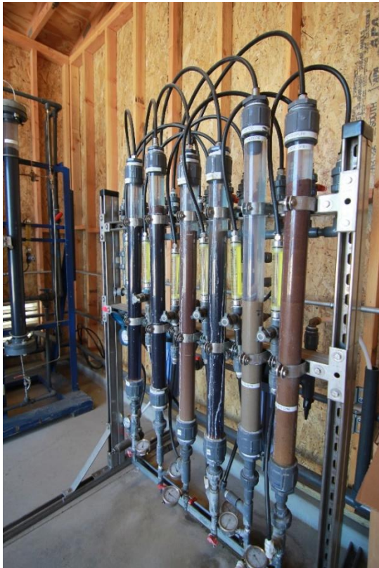
Figure 7. IX and alternative adsorbent pilot skid (left) and closer view (right) showing color of four IX resins at the beginning of the pilot test
