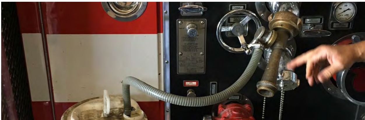
Figure 6. Idaho National Laboratory fire truck AFFF eductor spray mechanism.
