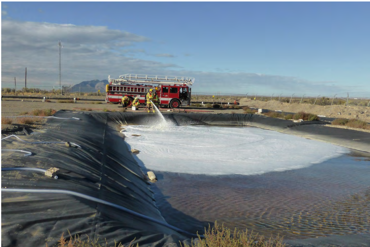
Figure 7. AFFF sprayed to contaminate lagoon water.
