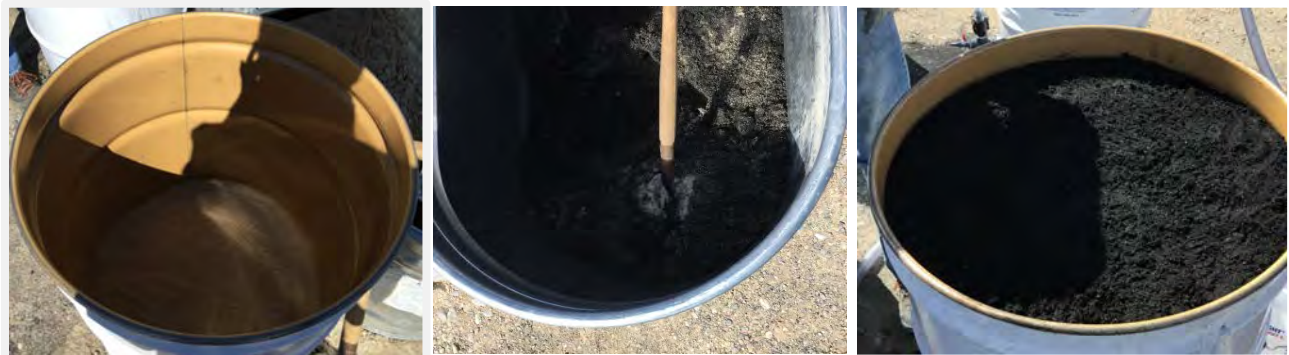
Figure 5. Rembind™ media mixed with sand.
