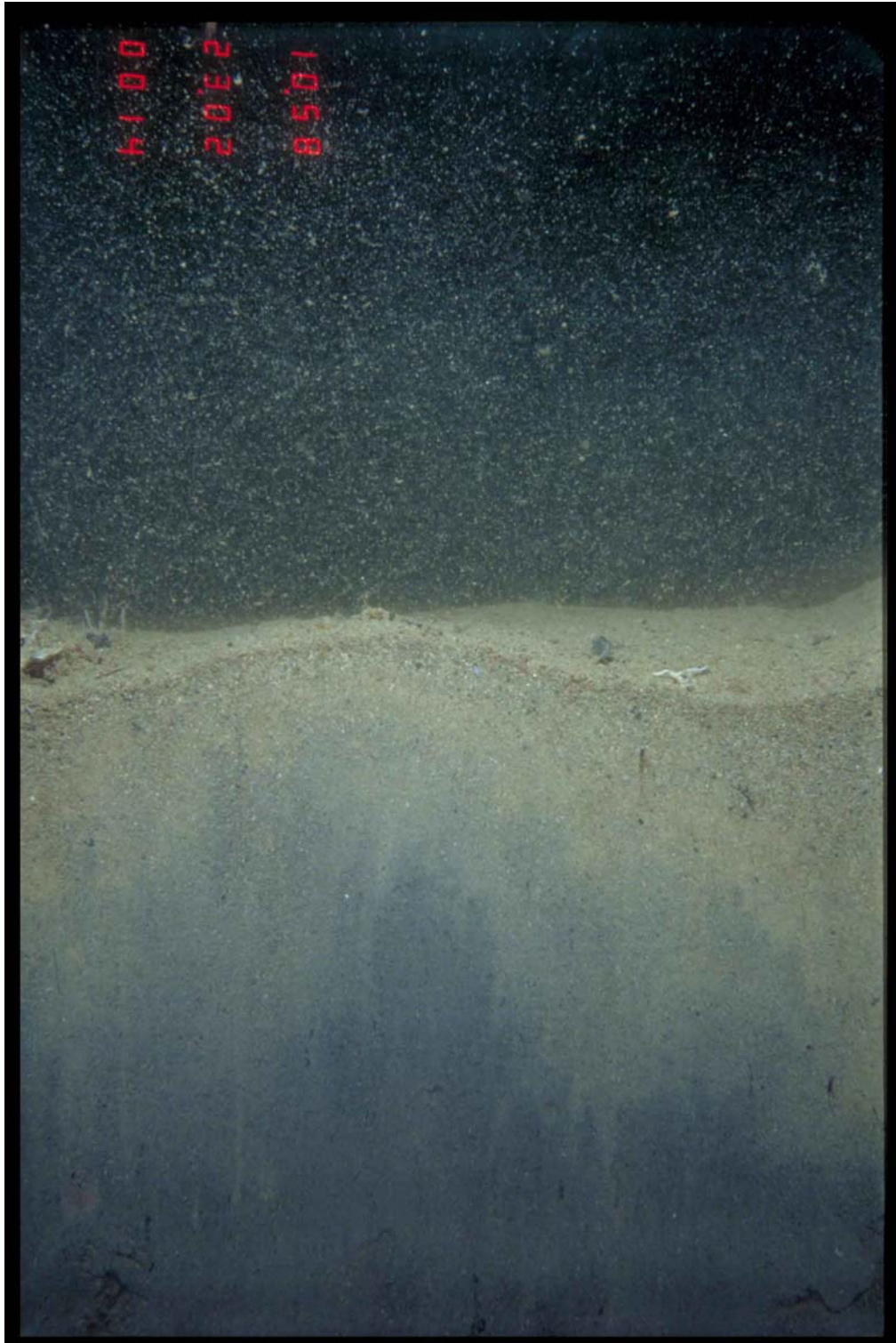
Figure 5-4. Sediment profile image from Station B at Bishop Point; a distinct accumulation of fine carbonate sands can be seen in the surface sediment (Scale: Width of image=15 cm).
