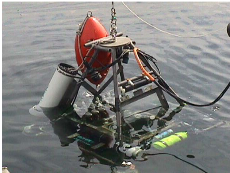
Figure 5-29. The Benthic Flux Sampling Device (BFSD2) used to sample sediment fluxes at Pearl Harbor.
