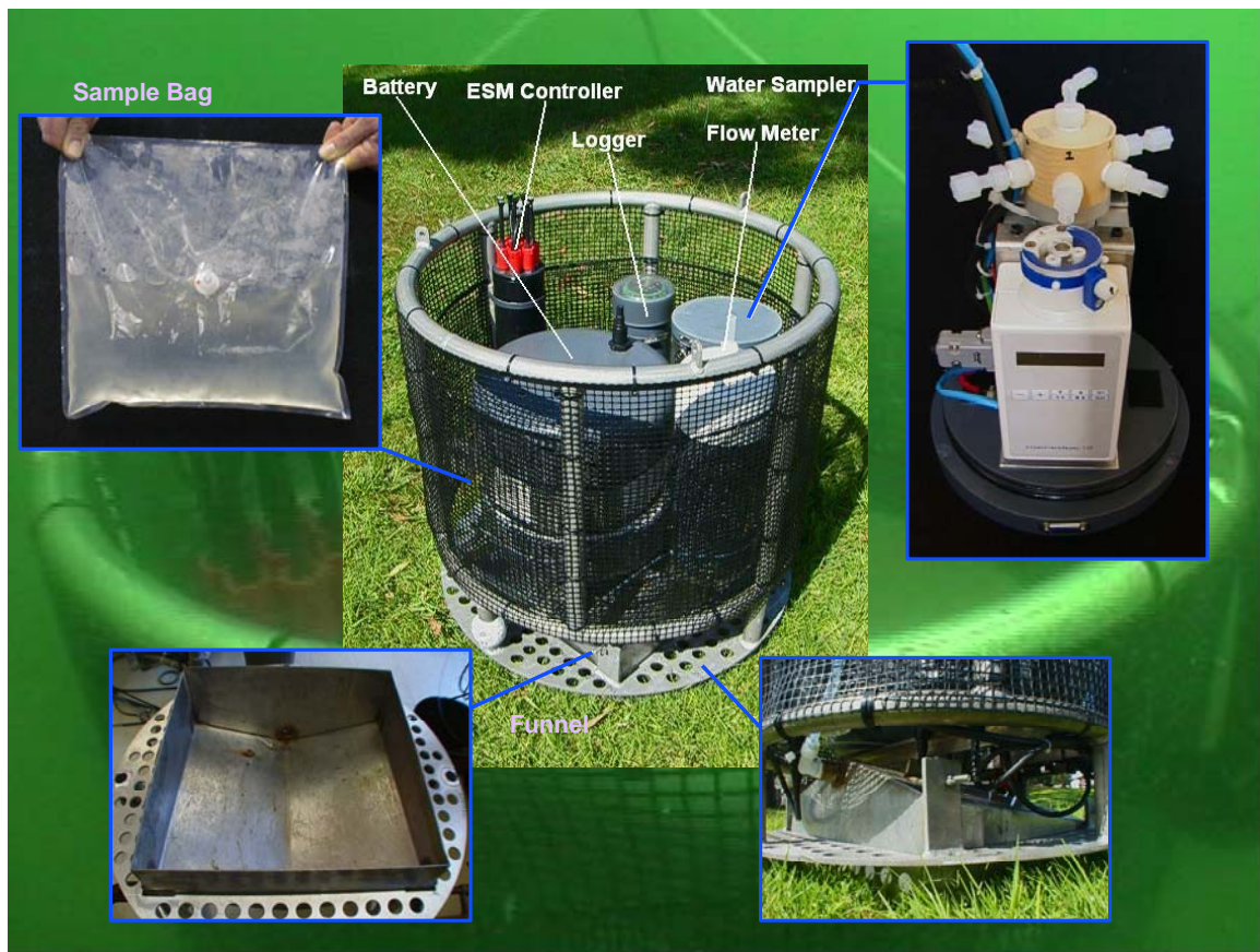
Figure 5-58. Component view of the prototype UltraSeep showing the water sampling and control units, battery housing, flow meter, data logger and funnel.
