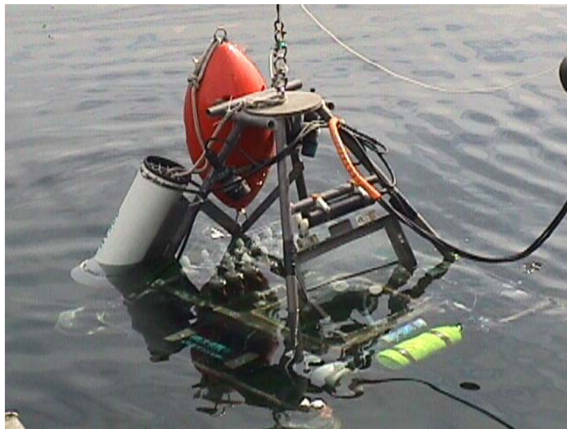
Figure 5-24. The Benthic Flux Sampling Device (BFSD2) used to sample sediment fluxes at Paleta Creek.
