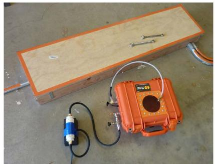
Figure 3.8. Photo of lung sampler (orange box) next to a monitoring location.
