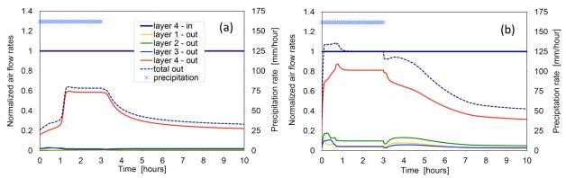
**Figure 5.15.** Transient change in airflow rates (a) Rainfall experiment (b) Heat experiment. These are comparable to Figures 5.9 and 5.11, respectively. Air leaving through the surface is the area above the total out, air confined within subsurface is below the total out.
