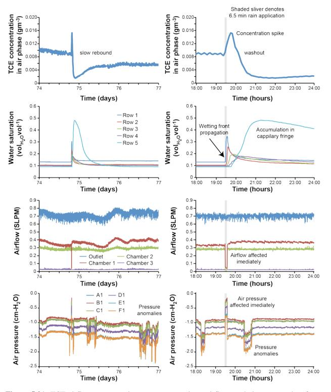
**Figure 5.21:** TCE airflow concentrations, water saturations, airflow, and air pressure data from rain event 2 (R2). Left column shows data from the wider timescale of the 3 full days surrounding the rainfall event. Right column presents the same data at higher temporal resolution, showing the 1.5 hours leading to the rainfall event, and 4.5 hours after the rainfall.
