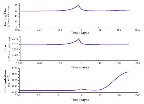
Figure 5.52: Effect of infiltration at 1 mm/hr for 24 hours on vapor signals in sandy clay loam scenario.
