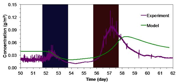
**Figure 5.30:** Comparison of experiment and model for TCE concentrations at tank outlet. Blue shaded region represents rising water table interval and pink shaded region indicates falling water table.
