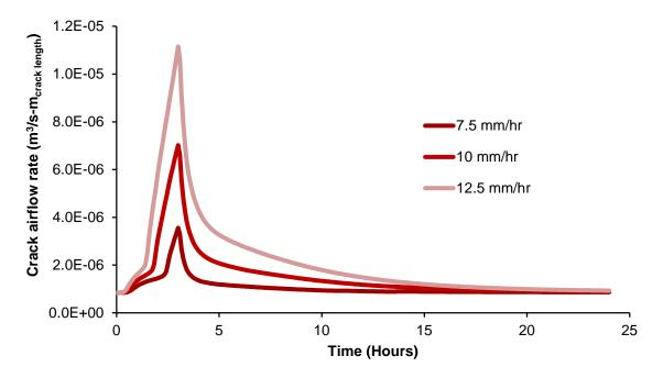
**Figure 5.51:** Scenarios showing effect of precipitation rate on airflow rate into building. Simulation was for sandy clay loam soil with a water table at 10m depth, and 5 Pa indooroutdoor pressure differential.
