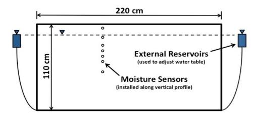
**Figure 4.12:** Schematic of the geophysical tank experiment apparatus with reservoirs used to control water table elevation and moisture sensors installed along a vertical profile. Moisture sensors were installed at vertical elevations of 4, 14, 25, 30, 35, 40, and 55 cm bgs (below ground surface). Total volume of sand tank apparatus is 163,350 cm<sup>3</sup>.
