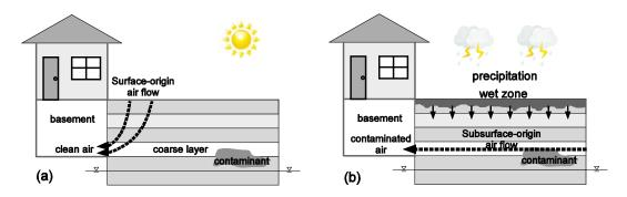
**Figure 5.16.** Schematic images of air flow pathway dynamics under different climatic conditions at the soil surface; (a) surface-origin air flow with small area of influence under no rainfall conditions, (b) subsurface-origin air flow with larger area of influence under rainfall conditions.
