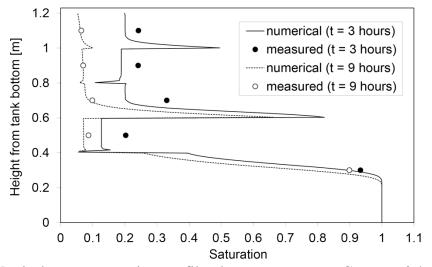
**Figure 5.12.** Vertical water saturation profile along sensor array C at t = 3 hours (when the rainfall stopped) and at t = 9 hours. Note that the larger the contrast at the fine-to-coarse interface, the higher the water saturation above the interface that leads to more significant capping effect.
