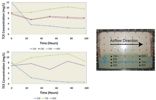
**Figure 5.7:** Aqueous TCE concentrations in the capillary fringe from experiment 3. Tank diagram at right shows locations of sample points. Water phase is dyed green for ease of viewing, while the vadose zone above the fringe appears as clean sand.
