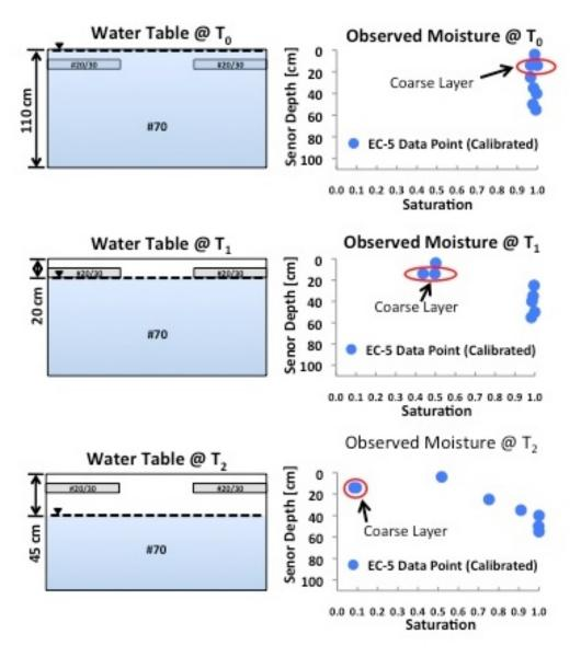
**Figure 5.35:** Schematic of packing configuration #2 and the calibrated volumetric moisture content data (e.g. Sakaki et al., 2011) with the water table set at the upper, mid and lower elevations (T0, T1, and T2, respectively).
