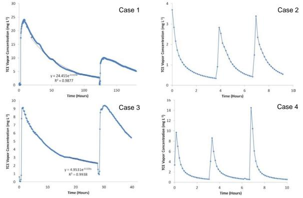
Figure 5.6: Effluent vapor concentration over time for all 4 cases. Spikes indicate separate experiments where the system is stopped, re-saturated, drained and resumed.
