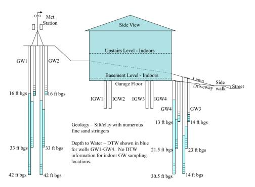
**Figure 4.17:** Schematic of water table elevations across field demonstration site [*Ongoing VI site study by Johnson et al.*, 2010-2012].
