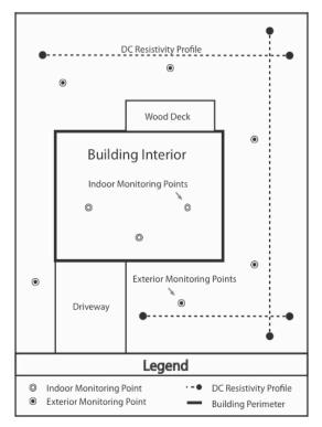
**Figure 4.15:** Schematic of VI monitoring locations with exterior and interior monitoring points indicated by concentric circles (oxygen concentrations, pressure potential, and soil gas sampling ports) and ERT profiles indicated by dashed lines with solid circular ends.
