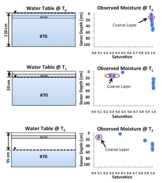
**Figure 5.34:** Schematic of packing configuration #1 and the calibrated volumetric moisture content data (e.g. Sakaki et al., 2011) with the water table set at the upper, mid and lower elevations (T0, T1, and T2, respectively).
