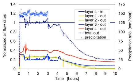
**Figure 5.11.** Air inflow and outflow rates and precipitation rate (Heat experiment). Precipitation was stopped and heat was turned on at t = 3 hours. "Total out" is the sum of the outflow rates from layers 1 through 4. Air leaving through the surface is the area above the total out, air confined within subsurface is below the total out.
