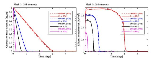
**Figure 4:** TCE concentration (left column) and cummulative TCE content depletion (right column) temporal profiles obtained using the C++ code using the NumDwarf library (solid line) compared to computational model built using COMSOL Multiphysics software version 3.5a (dashed line).
