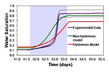
**Figure 5.31:** Comparison of water saturations at array 5 for the hysteresis model, non-hysteresis model and data for the water table rise.
