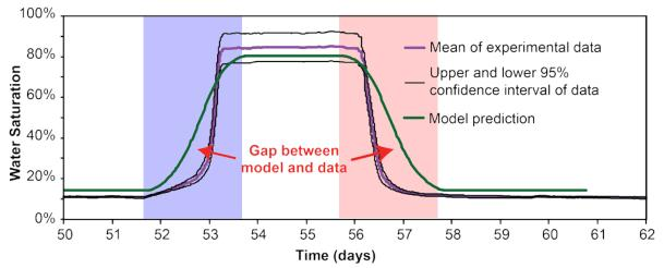
**Figure 5.29:** Model and experimental comparison of mean soil moisture values in array 5 during the water table fluctuation event. Blue time period corresponds to rising water table and pink time period corresponds to the dropping water table.
