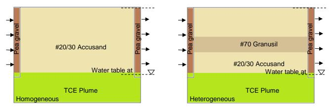
**Figure 4.4:** Capillary fringe volatilization experiments packing configuration and cases 1-4 description
