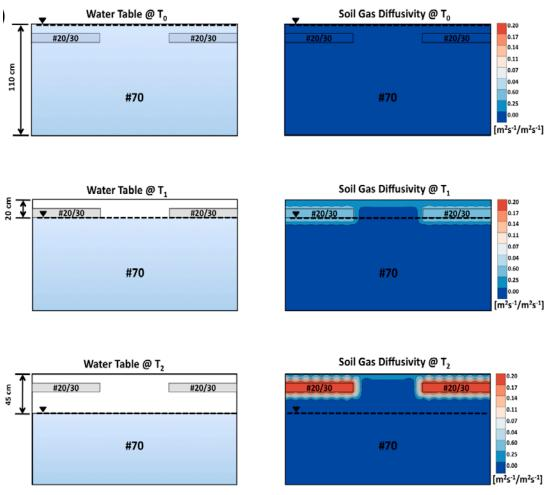
**Figure 5.38:** Schematic of packing configuration #2 and the soil gas diffusivity simulations (Moldrup et al., 2000) with the water table set at the upper, mid and lower elevations (T0, T1, and T3, respectively).
