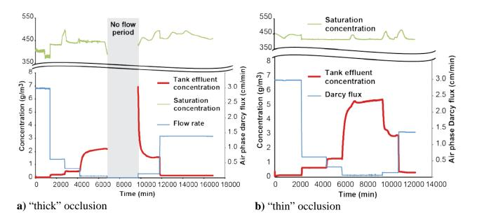
**Figure 5.1**: Measured TCE effluent vapor concentration versus time for a) the 13.8 mm "thick" occlusion and b) the 8.5 mm "thin" occlusion. The red line represents the concentration of TCE in the effluent soil gas (g/m3), green line represents the saturation concentration of TCE estimated from temperature data using values from Boublík et al. (1973)(g/m3) (note y-axis break), and the blue line represents the air phase Darcy flux in the unsaturated portion of the tank.
