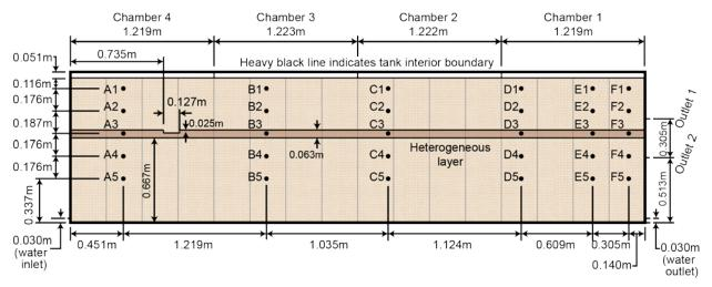
Figure 4.10: Detailed schematic of tank design and configuration.
