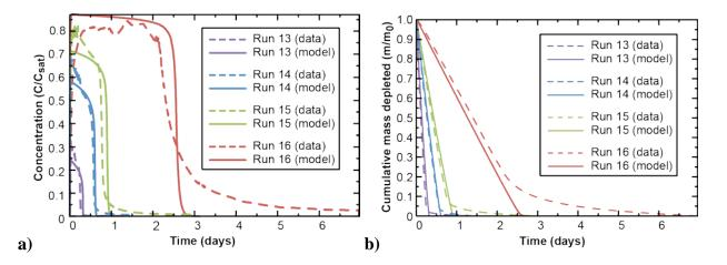
**Figure 5.4:** Concentration versus time for exposed source NAPL systems (a), the model (solid line) and measured data (dashed) outflow concentrations and (b) the model (solid line) and measured data (dashed) mass depletion curves.
