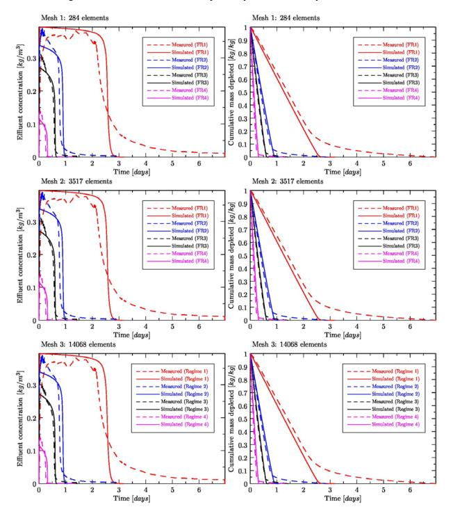
**Figure 2:** TCE concentration (left column) and cummulative TCE content depletion (right column) temporal profiles compared to laboratory measured data (dotted lines) for the best fitted parameters during the four fitting parameters procedure (Section 5.1) given in the second row in Table 2.
