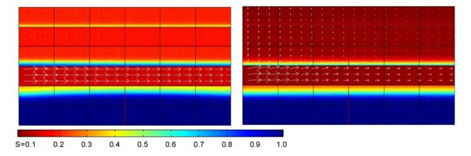
**Figure 5.13.** Soil water saturation distribution and air flow field (left) t = 3 hours, (right) t = 9 hours. Note that most of the injected air flows through layer 4 at t = 3 hours due to high saturation at the capping interface (i.e., large area of influence), whereas a significant portion passes through the capping interface at t = 9 hours and the flow in layer 4 diminishes over distance (i.e., small area of influence).
