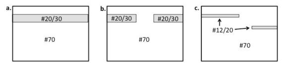
**Figure 4.13 (a-c).** Schematic of geophysical sand tank packing configurations: (a) *Configuration* #1 – Fine matrix (#70 sand) with coarse continuous horizontal layer (#20/30 sand, 10 cm. thick). (b) *Configuration* #2 – Fine matrix (#70 sand) with coarse discontinuous horizontal layer (#20/30 sand, 10 cm. thick). (c) *Configuration* #3 - Fine matrix (#70 sand) with shallow and deep thin discontinuous horizontal layers (#12/20, 4 cm. thick). Figures not drawn to scale.
