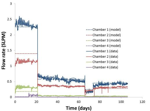
**Figure 5.26:** Simulated vs. observed data for airflow rates in the 4 flux chambers (units = standard liters per minute). Flux chambers are numbered 1-4 with decreasing proximity to the air outlet (see figure 4.10).
