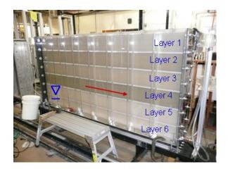
Figure 4.8: Photo of the two-dimensional tank apparatus.
