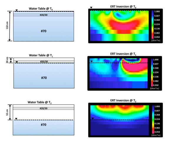
**Figure 5.40:** Schematic of packing configuration #1 and the ERT inversions with the water table set at the upper, mid and lower elevations (T0, T1, and T3, respectively). The ERT inversion color gradients represent resistivity values with ranges from 0.05 Ohm\*m to 1.00 Ohm\*m.
