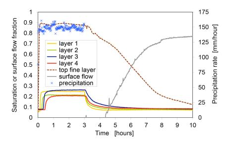
**Figure 5.10.** Soil water saturation and surface flow fraction (Heat experiment). The surface flow fraction was obtained based on the difference between the inflow and the total outflow from the four layers. Precipitation was applied for 0 < t < 3 hours, heat was applied for 3 < t < 10 hours.
