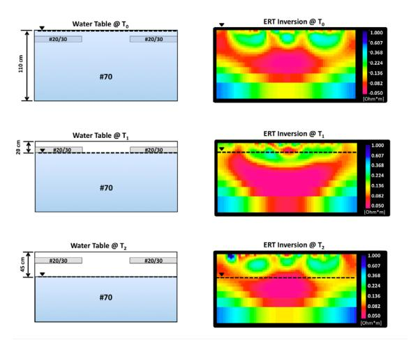
**Figure 5.41:** Schematic of packing configuration #2 and the ERT inversions with the water table set at the upper, mid and lower elevations (T0, T1, and T3, respectively). The ERT inversion color gradients represent resistivity values with ranges from 0.05 Ohm\*m to 1.00 Ohm\*m.
