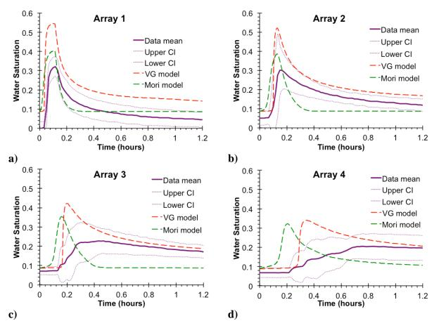
**Figure 5.27:** Water saturation profiles for model(s) and experimental data as a function of sensor array elevation. Sensor arrays increase in depth from 1 to 4, showing the propagation of the wetting front with time. Shown also are the 95% confidence intervals for the mean.
