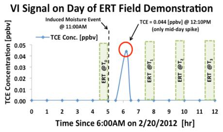
**Figure 5.47:** Graph of the VI signal (TCE in ppbv) entering study site building over 1-day window during our ERT field demonstration with ERT time-series snap shots overlaid on the VI signal timeline [Ongoing VI site study by Johnson et al., 2010-2012].
