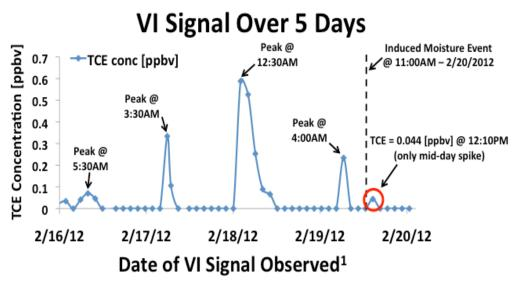
**Figure 5.46:** Graph of the VI signal (TCE in ppbv) entering study site building over a five-day window that included our field demonstration and simulated precipitation event. [Ongoing VI site study by Johnson et al., 2010-2012].
