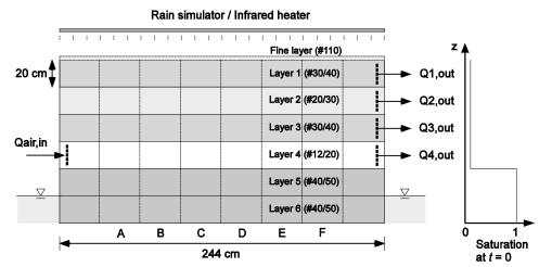
**Figure 4.7:** Schematic view of the two-dimensional tank for dynamic soil moisture experiments. Saturation profile is only schematic. Note that the air flow is reversed in the rainfall and heat experiments.
