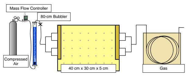
Figure 4.3: Schematic of capillary fringe volatilization experimental apparatus
