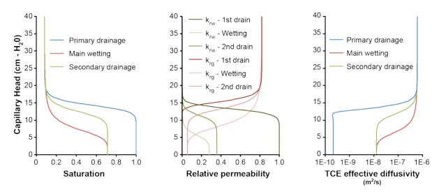
**Figure 5.5:** Estimated van Genuchten saturation, Mualem air and water relative permeability and Millington-Quirk effective diffusivity curves for the 20/30 Accusand used in the study. Included are curves for primary drainage cycle, main wetting cycle, and the secondary drainage cycle. Note logarithmic axis for diffusivity curves.
