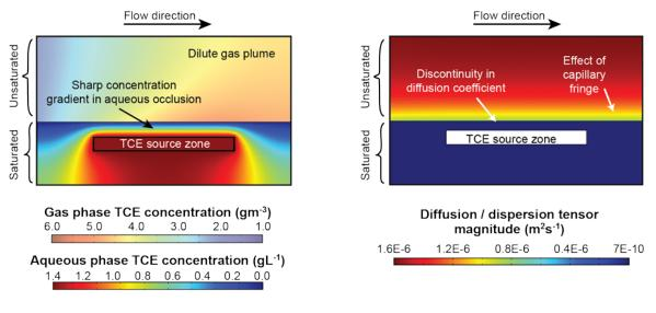
**a**) Concentration profile: pastel scale shows gas phase concentrations, dark axis shows aqueous concentrations
