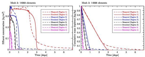
**Figure 3:** TCE concentration (left column) and cummulative TCE content depletion (right column) temporal profiles compared to laboratory measured data (dotted lines) for the best fitted parameters during the three fitting parameters procedure (Section 5.2) given in the fourth row in Table 2.
