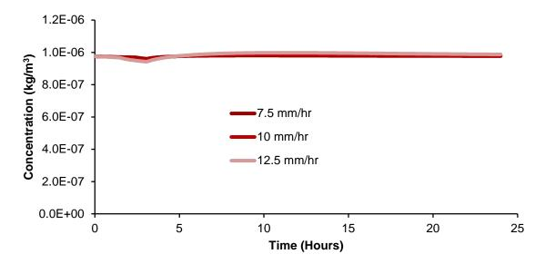
**Figure 5.50:** Effect of rainfall intensity on TCE concentrations of soil gas entering the building for the silty clay loam soil.
