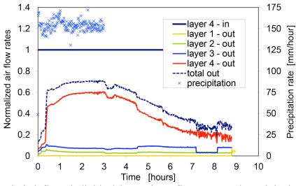
**Figure 5.9.** Total air inflow, individual layer air outflow rates and precipitation rate (Rainfall experiment). "Total out" is the sum of the outflow rates from layers 1 through 4. Air leaving through the surface is the area above the total out, air confined within subsurface is below the total out.
