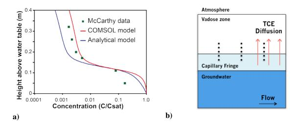
**Figure 5.24:** a) COMSOL model compared against McCarthy and Johnson (1996) data and analytical model. Note that the error bars for McCarthy and Johnson data are smaller than the data marker. Note logarithmic concentration axis. b) diagram of McCarthy and Johnson experimental apparatus (1 m x 1 m).
