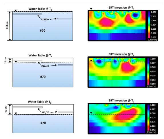
**Figure 5.42:** Schematic of packing configuration #3 and the ERT inversions with the water table set at the upper, mid and lower elevations (T0, T1, and T3, respectively). The ERT inversion color gradients represent resistivity values with ranges from 0.05 Ohm\*m to 1.00 Ohm\*m.
