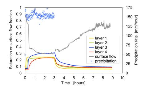
**Figure 5.8.** Soil water saturation by layer and total surface flow fraction (Rainfall experiment). The surface flow fraction was obtained based on the difference between the inflow and the total outflow from the four layers. Precipitation was applied for the first 3 hours.
