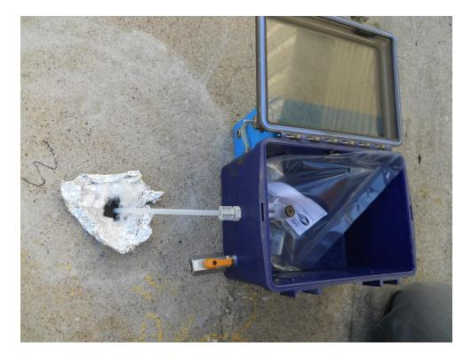
Figure 19: Vacuum chamber used to purge subslab probes prior to passive sampler deployment
