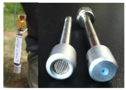
Figure 2e: ATD tube sampler and regular and low-uptake rate caps
