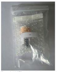
Figure 1: WMS<sup>™</sup> sampler with glass overpack vial, unsealed bubble pack and plastic bag.
