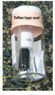
Figure 2: Close-up of WMS<sup>™</sup> sampler in its glass overpack shipping vial
