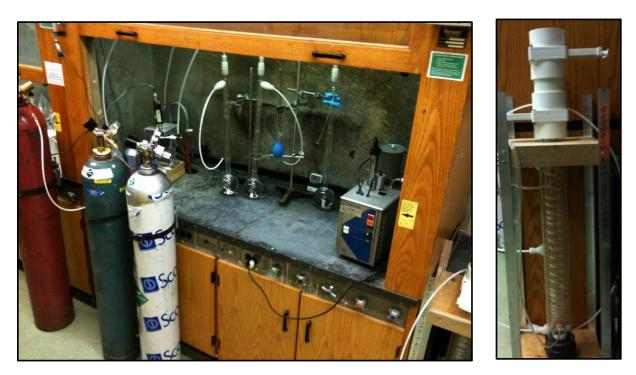
**Figure 14:** Photograph of high concentration laboratory experimental apparatus, showing (left to right: nitrogen cylinder, cylinders with VOC mix, mass flow controller, humidification vessels, temperature bath (on left) and the exposure chamber (on right))
