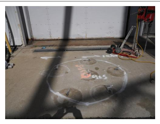
Figure 18: Sub-slab probe array (OTC3)
