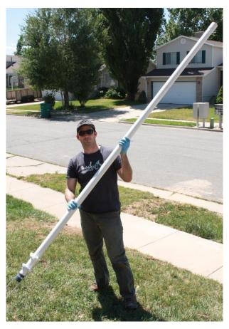
Figure 22: Photograph of passive soil vapor probe before installation
