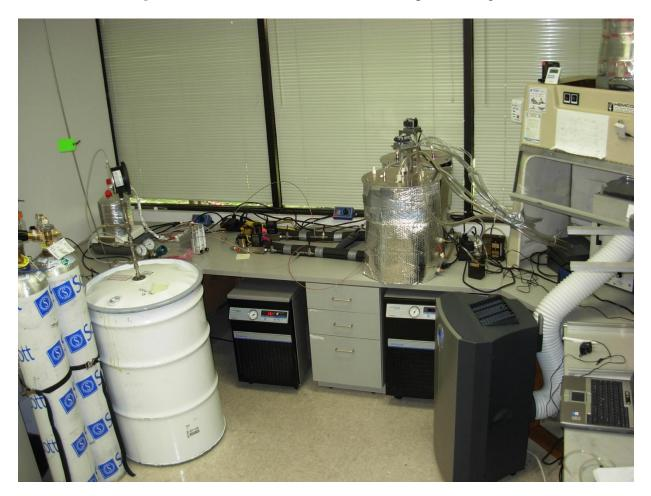
**Figure 12:** Low concentration test apparatus, including (left to right: compressed gas cylinders containing 10 VOCs, drum of activated carbon for purifying dilution air, humidification vessel, mass flow controllers, exposure chambers (covered with insulation), constant temperature bath, and discharge lines to fumehood).
