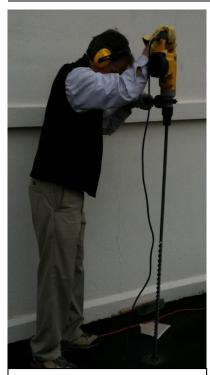
**Figure 27:** Installation of temporary passive soil vapor probe using hammer-drill and 1-inch diameter, 5-ft long drill bit at NAS JAX.
