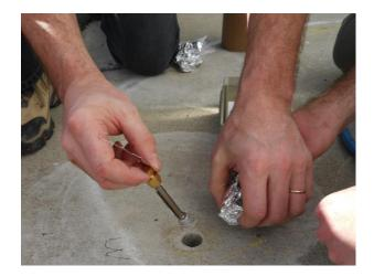
Figure 20: Deployment of a passive ATD tube sample
