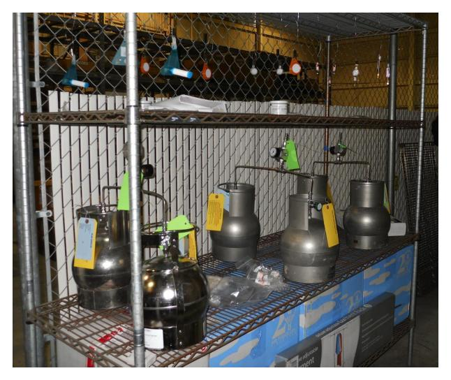
Figure 15: Typical layout of indoor air sampling array
