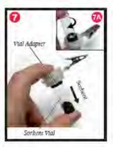
Mark sample vial as appropriate and insert into the pouch. Carefully package sample vial and a blank sorbent vial. Send to a laboratory for analysis.
