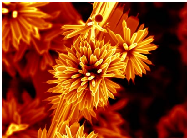
Figure 18. Zinc oxide nanostructures synthesized by a vapor-solid process.
