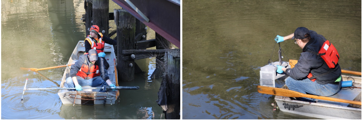
Figure 2a. Left: Sediment cores being collected from Segment 1 of A-Street Ditch. Right: Sediment porewater and surface water passive samplers being placed in Segment 1 of A-Street Ditch (March 14, 2019).
