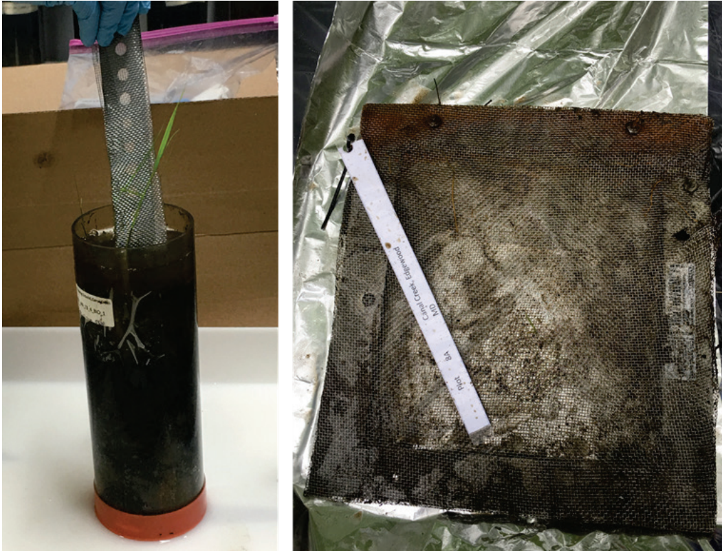
Figure 16. Passive samplers used at Canal Creek. Left: Ex situ pore water measurement within intact cores take from the Canal Creek site. A passive sampling strip enclosed in stainless steel mesh is shown being inserted into the core. Right: In situ passive sampler retrieved from the field. The passive sampling sheet was enclosed in a stainless steel mesh and frame.
