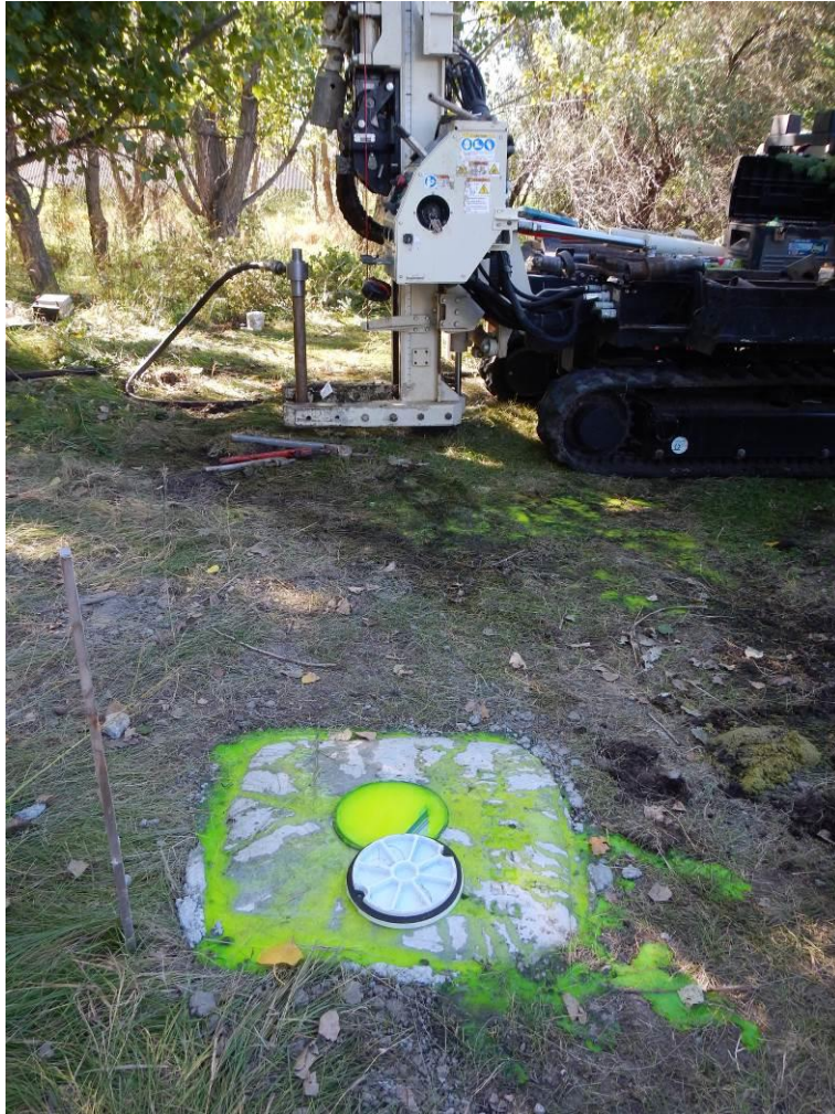
Photo 5 – Fluid Surfacing from MW17
