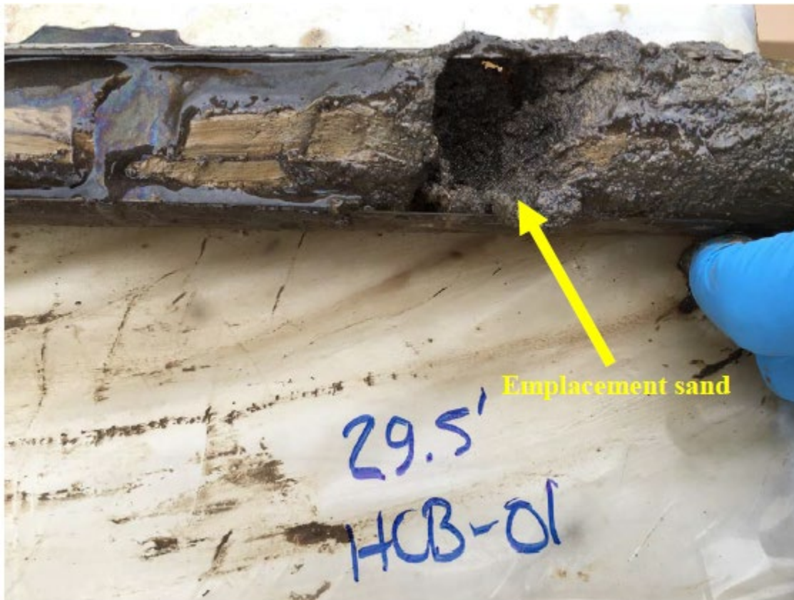
Figure 6.4. Visual Observations of Emplaced Silica Sand at Confirmation Boring HCB-01 within the Hydraulic Demonstration Cell at LCAAP
