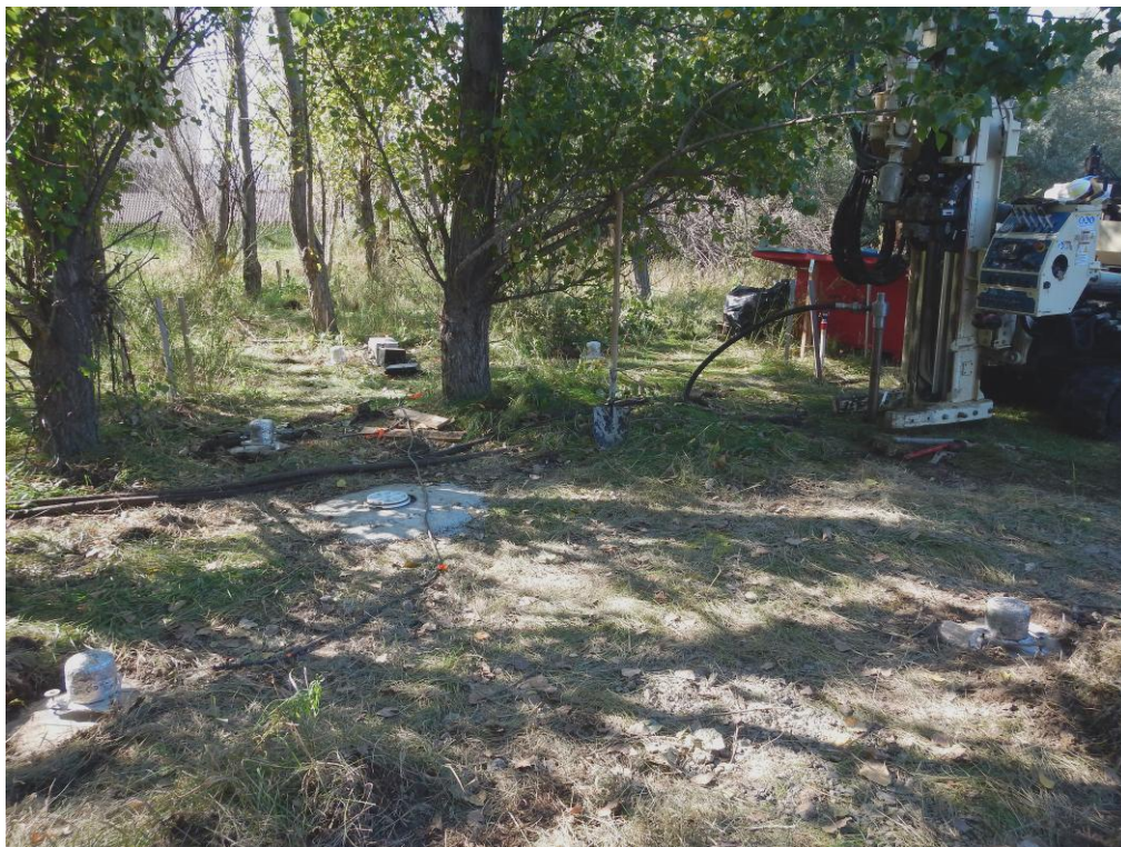
Photo 4 – Tiltmeters Placed Around HIP-01
