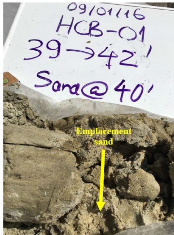
Figure 6.1. Visual Observations of Emplaced Silica Sand at Confirmation Boring HCB-01 at MCB-CP
