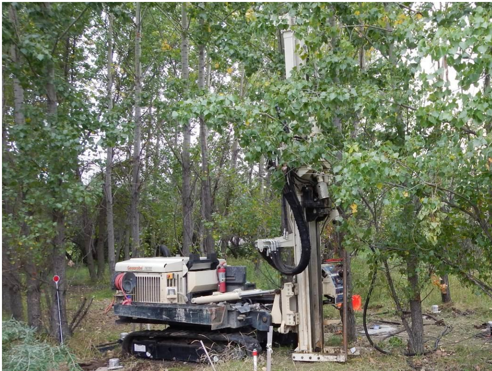
Photo 2 – Plain's Track Mounted Direct Push Drilling Rig
