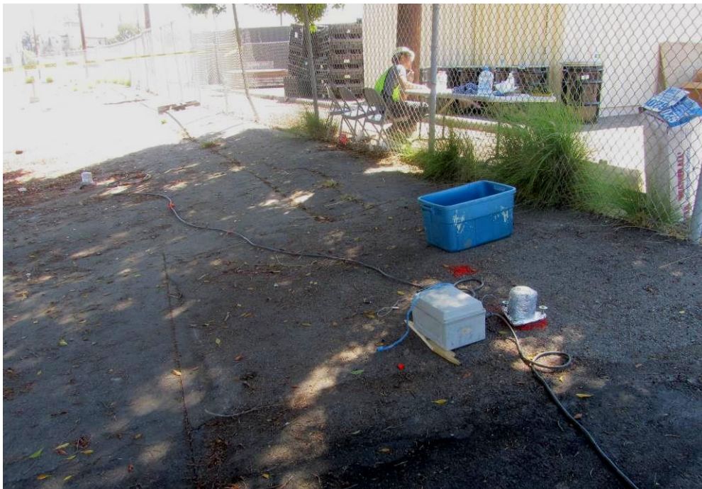
Photo 4 – Tiltmeters Placed Around HIW-01
