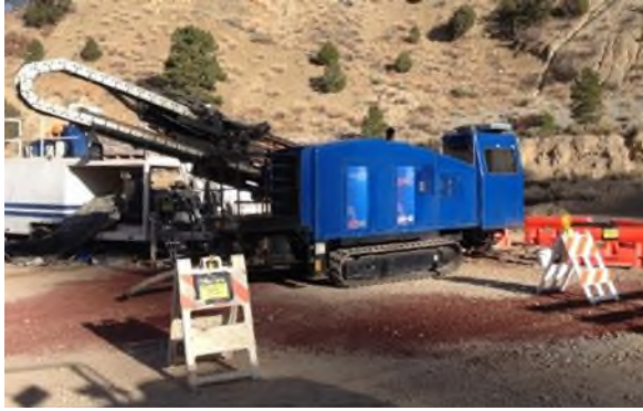
Figure 20. Directional Drilling Rig and Drill Bit
