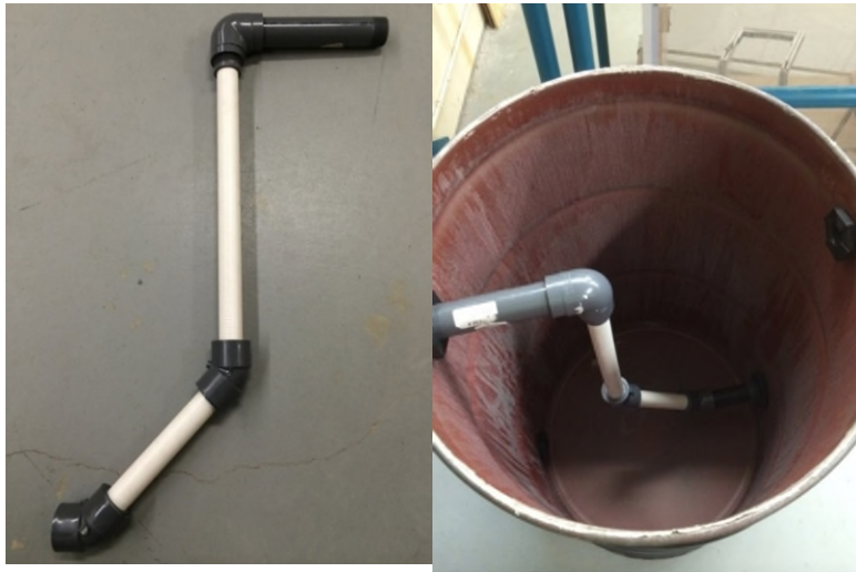
Figure 9. Laboratory Tank System Photographs of Laboratory Tank System with HRX Well constructed within a 55-gallon drum to simulate a simple aquifer system
