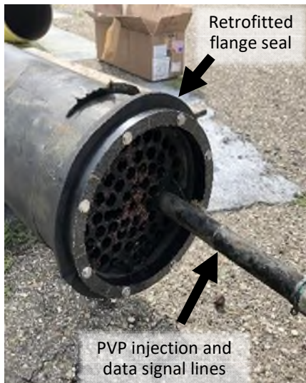
Figure 32. Photograph of Retrofitted Flange Seal on Monitoring Cartridge
