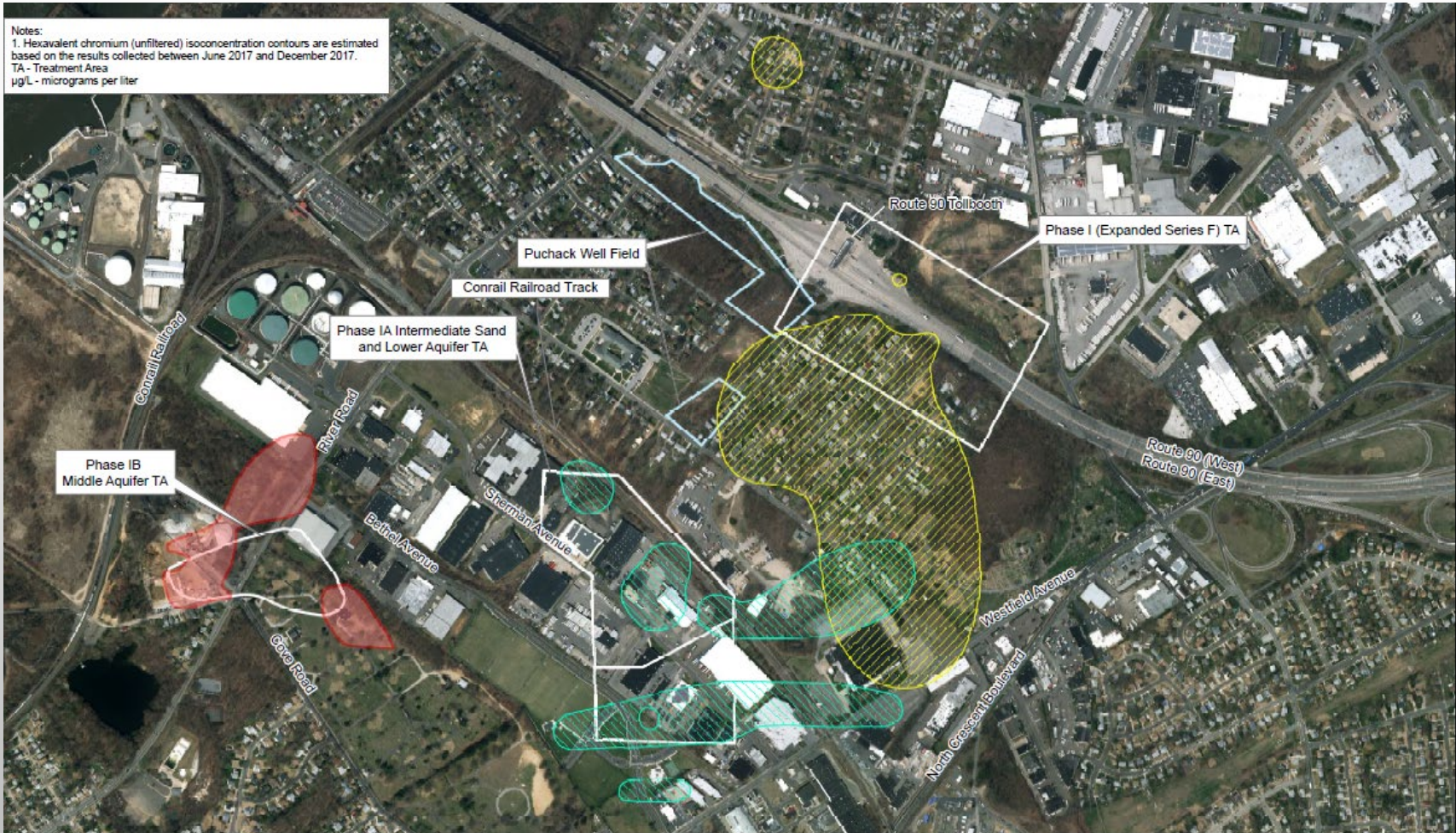
Figure 1-2 Phase I Actual and Phase II Proposed Remediation Areas Puchack Well Field Superfund Site - OU1 Pennsauken Township, New Jersey
