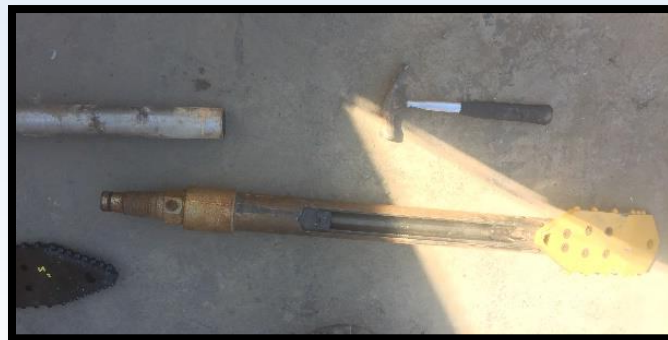
Drill bit housing with sonde
