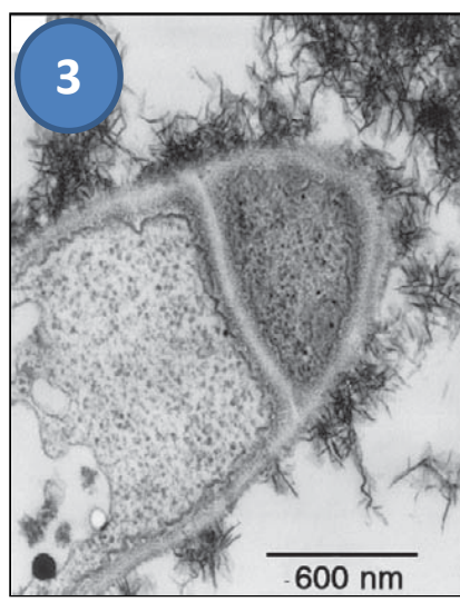
Biogenically synthesized manganese oxides (Miyata et al., 2007)
